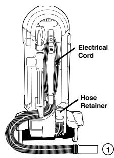
1. Remove hose from hose retainer and check suction at end of hose.
